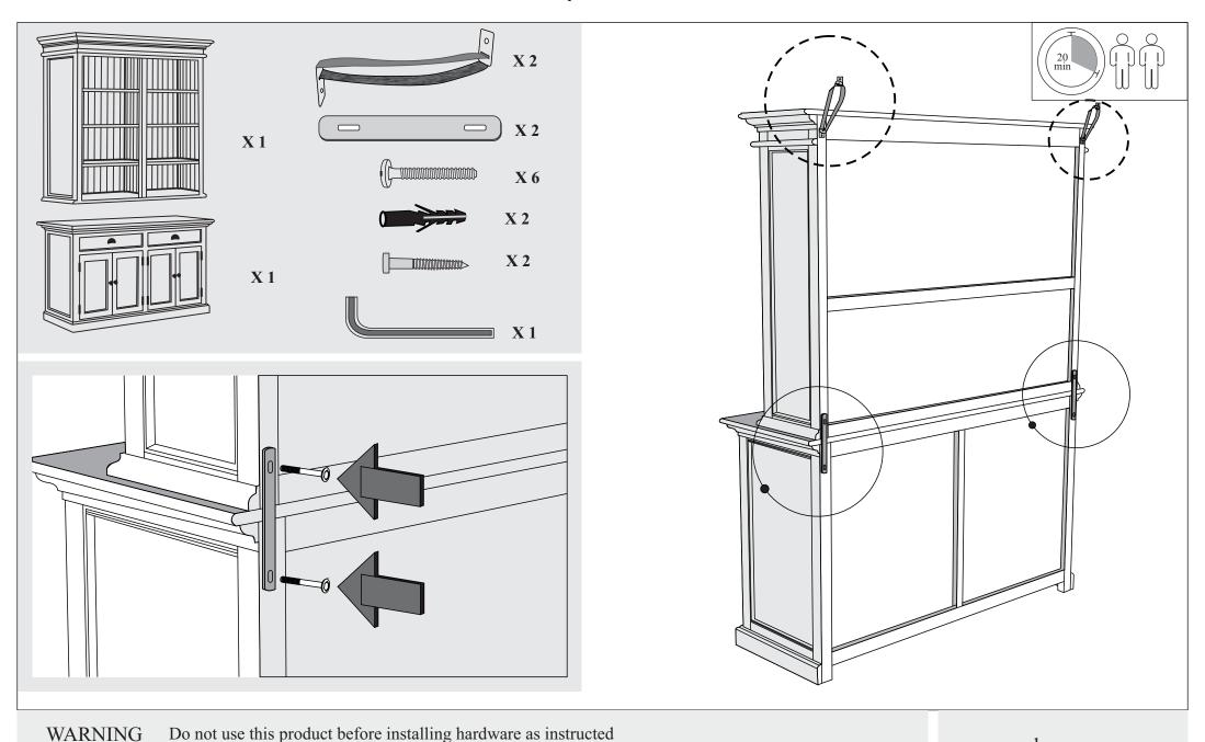
Do not use this product before installing hardware as instructed During assembly tighten screws by hand. Once all screws are in place use the tool to tighten until secure
